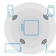
Smart Hub should be situated far from any metal obstacles, transformers, engines, fluorescent lamps, microwave devices, refrigerators and other industrial equipment.
