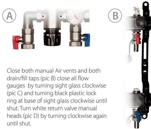
Close both manual Air vents and both drain/fill taps (pic B) close all flow gauges by turning sight glass clockwise (pic C) and turning black plastic lock ring at base of sight glass clockwise until shut. Turn white return valve manual heads (pic D) by turning clockwise again until shut.
