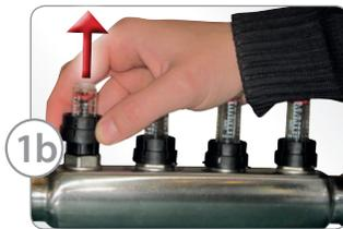
Turn flow gauge **anti-clockwise to open** and clockwise to close (pic 2b) the flow gauge is fully open when turned two full turns from closed position, do not force pass 2 full turns. Re-fit black lock clip once adjusted.
