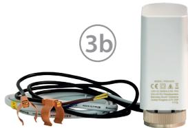
Each Auto Balancing actuator has two pipe sensors (pic 3b), one is simply clipped onto the flow and the other onto the corresponding return of each individual circuit. Either clip can be placed on the flow or return pipe (pic 4b)
