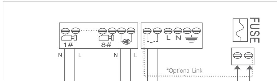
Max 3 actuators can be connected to one channel
