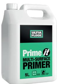
Prime It Multi-surface primer is used to prepare the aluminium surface of our EPS400 Overfloor boards prior to tiling directly onto using PROFLEX S2 tile adhesive. Applied neat to the entire surface of the aluminium, pipe and any exposed pipe channels – 1 tub = 50sqm coverage.
