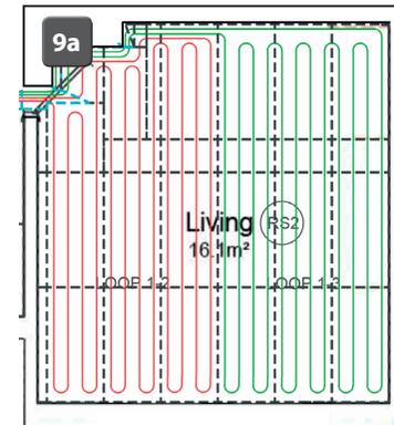
**9** Before laying pipe make sure all pipe channels are clear from debris, check and familiarise yourself with the pipe layout drawing (9a) plan where to begin and the pipe routes for each individual loop of pipe.
