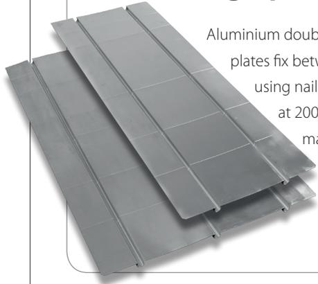
Aluminium double spreader plates fix between joists at 400mm spacing or triple spreader plates fix between joists at 600mm spacing. Designed for quick and simple installation using nails, screws or staples. Pipe is laid into the preformed omega channels at 200mm pipe centres. Insulation below the spreader plates will ensure maximum performance from this system.
