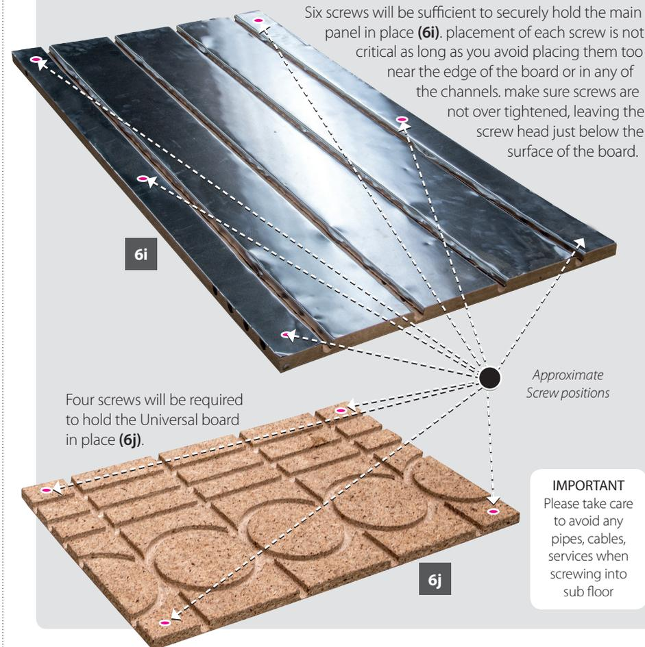
Six screws will be sufficient to securely hold the main panel in place (6i). placement of each screw is not critical as long as you avoid placing them too near the edge of the board or in any of the channels. make sure screws are not over tightened, leaving the screw head just below the surface of the board.
