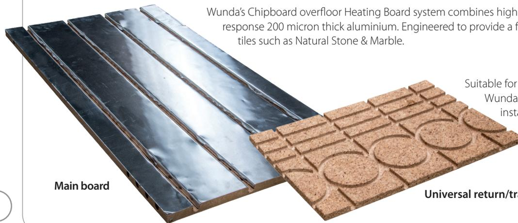
Wunda's Chipboard overfloor Heating Board system combines high compressive strength 17mm Chipboard with rapid response 200 micron thick aluminium. Engineered to provide a floor heating solution that can support heavyweight tiles such as Natural Stone & Marble.
