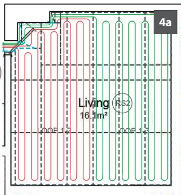
Before attempting to lay any floor heating boards, familiarise yourself with the system layout drawing, noting the manifold position. The drawing will detail the orientation and position of panels (4a).
