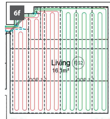
Working from the manifold location, start by laying end return and or transitional panels along one wall (6g) (working in conjunction with pipe layout drawing) (6f).
