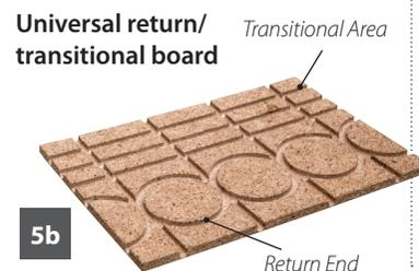
When cutting and creating new bends into a board, keep the radius gradual and no sharper than in a main panel. The water flow around a pipe circuit should always go to potential cold areas first, for example external walls and areas of high glazing. We suggest wearing flat soled shoes or trainers whilst walking on the boards.
